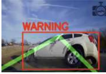
Fig. 4: Collision alert triggered by a vehicle cutting into the lane at close proximity
